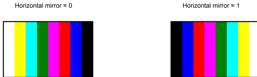
Figure 56: 100% Color Bars Test Pattern
