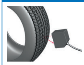
Measuring Tire Exteriors
