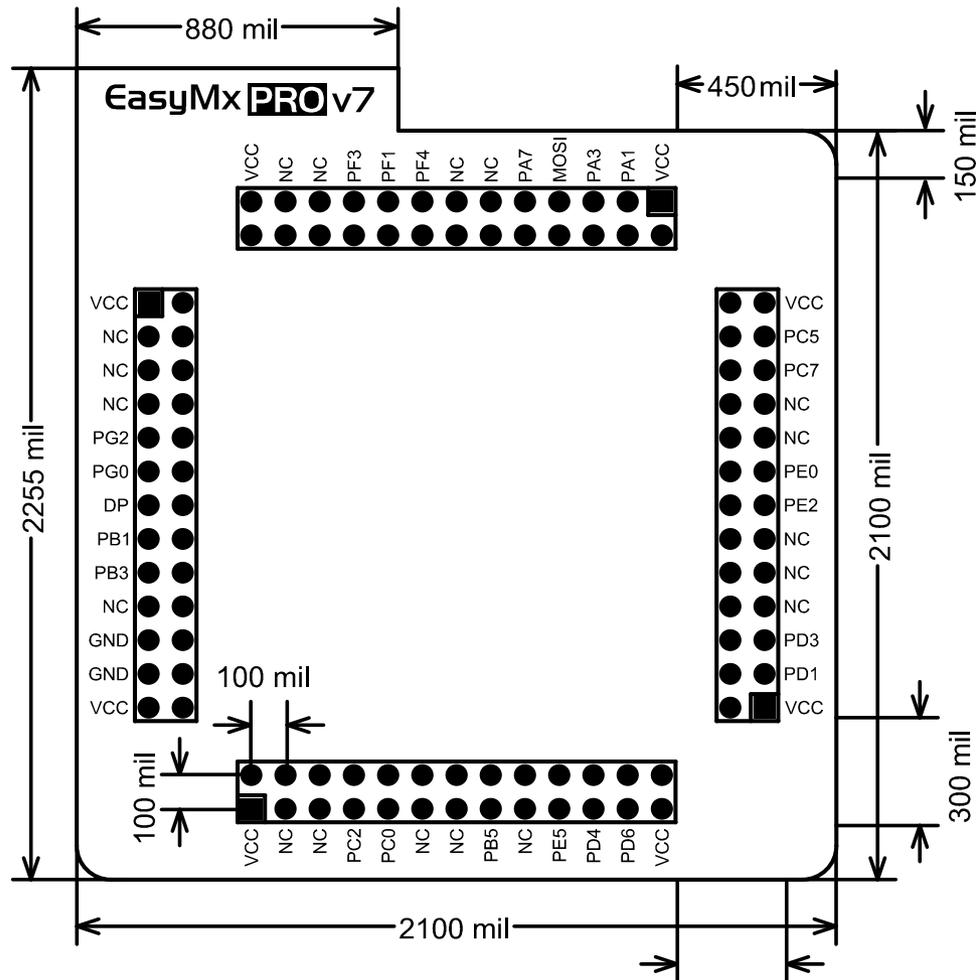
Figure 3: MCU card dimensions. Values are in mils.
