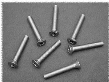
Part #: 1421F25 (package of 25) • 10-32 x 1.25" • Phillips oval head screws • Nickel plated
