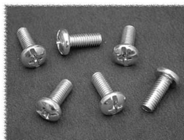
Part #: 1421D (package of 25) • 10-32 x 0.5" • Slotted & phillips combination pan head screws • Use where economy is important OR for close panel spacing. • Zinc plated
