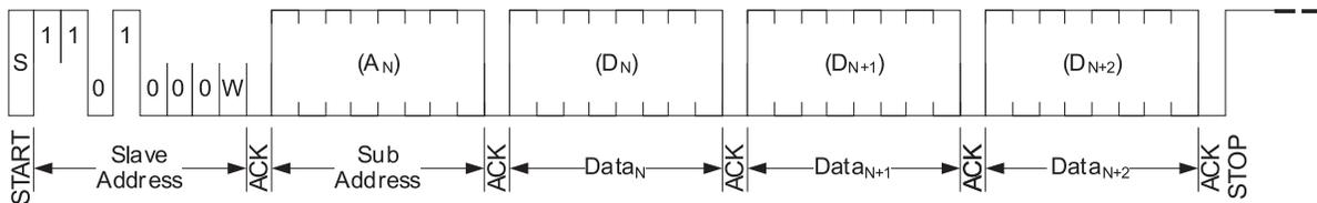
**Figure 5. I<sup>2</sup>C Write Mode**
