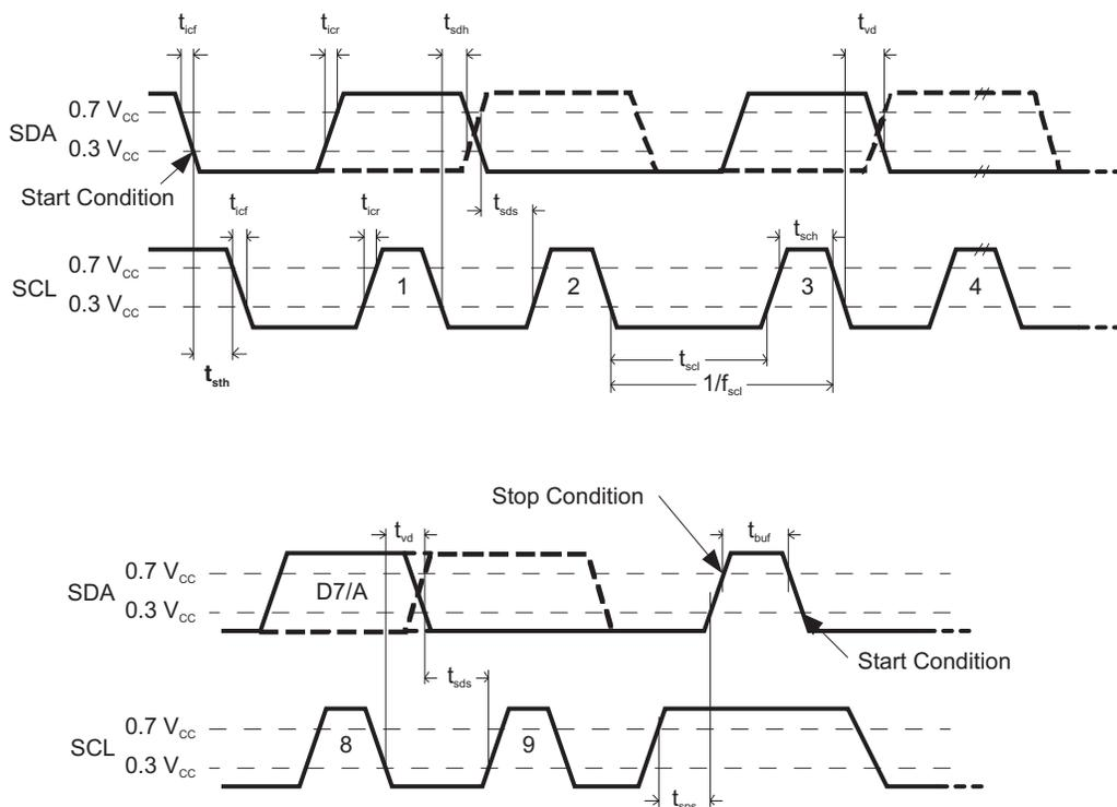
Figure 3. I<sup>2</sup>C Timing Diagram
