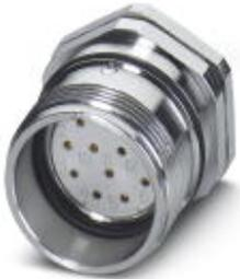
Device connector with M20 x 1.5 screw-in thread, straight, shielded: yes, Screw locking, M23, No. of pos.: 6, type of contact: Socket, Crimp connection, Axial O-ring, Central fixing, Panel thickness min.: 0.8 mm, Panel thickness max.: 6.5 mm
