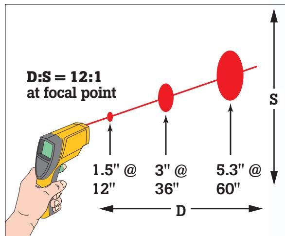
Use the Fluke 63 within six feet of the intended target. At greater distances, the measured area will be larger (approximately the distance divided by 12). The Fluke 63 offset single-point laser indicates the approximate center of the measurement area.
