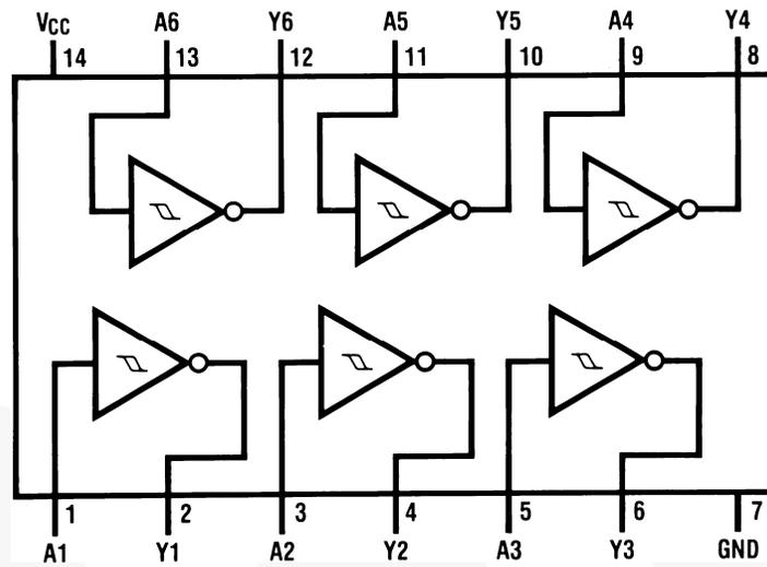
Figure 1. Pin Assignments
