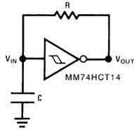
Figure 3. Low Power Oscillator
