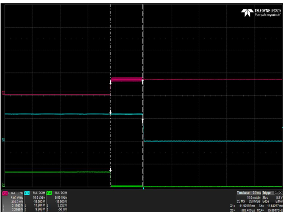
Figure 11: DS1600SPE-3 Turn Off Characteristic via PS_ON_L Full Load: I_o = 129.8A , I_{sb} = 3.5A Ch 2: PS_ON_L Ch 3: Vo Ch 4: Pwr_Good
