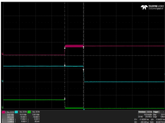
Figure 11: DS1600SPE-3 Turn Off Characteristic via PS_ON_L Full Load: I_o = I_o = 129.8A , I_{sb} = 3.5A Ch 2: PS_ON_L Ch 3: Vo Ch 4: Pwr_Good
