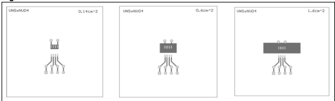
Figure 37. SO-8 PC board (1)
