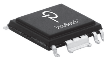
Figure 2. High Creepage, Safety-Compliant eSOP Package.
