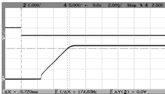
On/Off Enable Delay (Vin=12V, Vout=3.3V, Iout=6A, Cload=0) Trace 4=Enable, Trace 2=Vout
