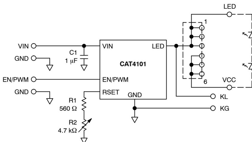
Figure 2. CAT4101AGEVB Board Schematic
