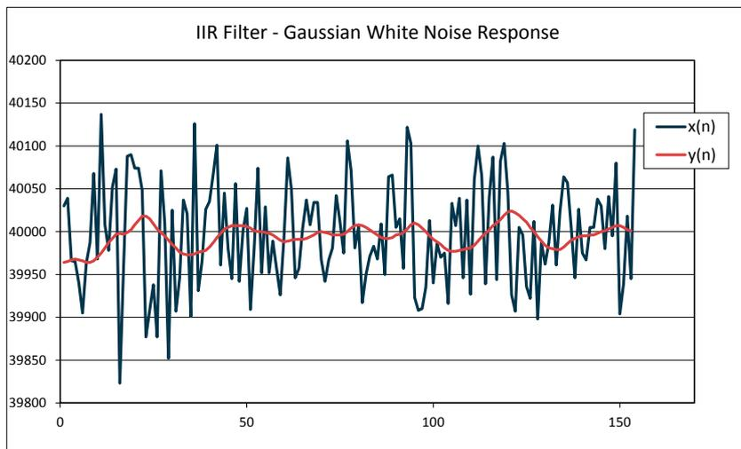
Figure 8 – Noise Response for the IIR Filter
