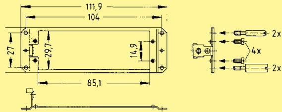
Retaining frame with 2 contact pins and ground termination
