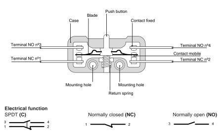
The NO and NC circuits must both be of the same polarity.
