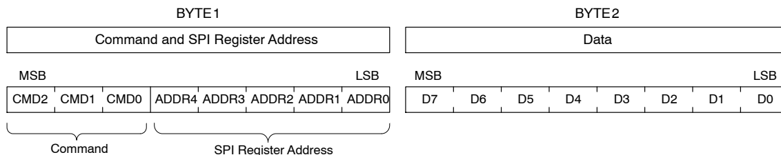
Figure 19. SPI Transfer Packet
