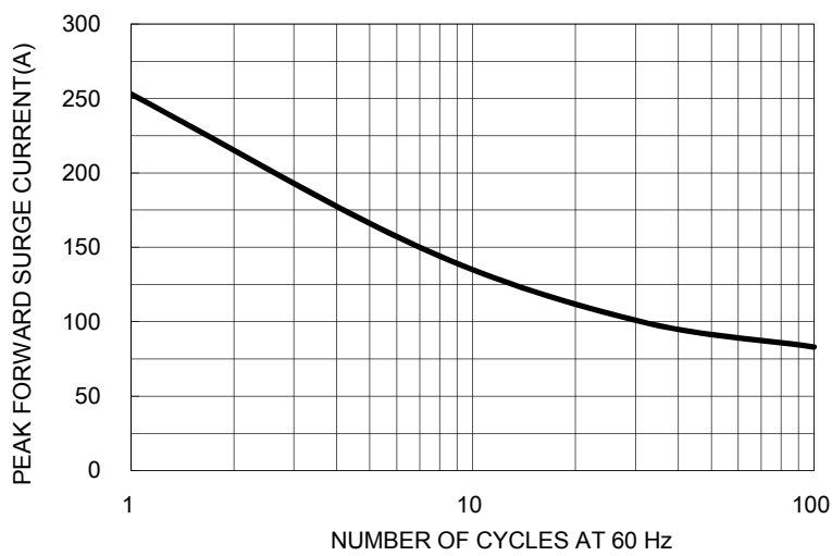
FIG. 3- MAXIMUM NON-REPETITIVE FORWARD SURGE CURRENT
