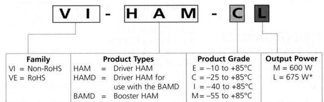
If power requirements exceed one HAM, use a HAMD and one or more BAMDs, with an external bridge rectifier. HAM, HAMD, and BAMD modules require three surge suppressors in series directly across the input. These surge suppressors are already contained in the EMI filter P/N 30205. Also use a 10A, 3AG fast-blow fuse ahead of the line filter.
