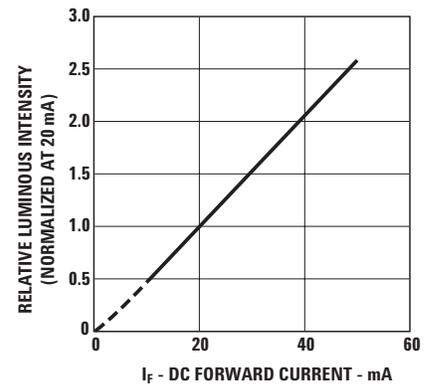
Figure 3. Relative Luminous Intensity vs. Forward Current
