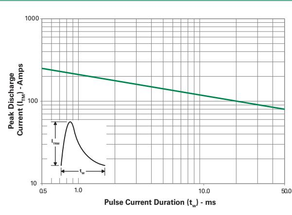
**Figure 12: Peak Capacitor Discharge Current Derating**
