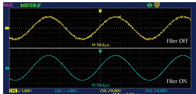
Filter out unwanted signal components such as various types of noise with built-in digital filters. Choose from Low-Pass, High-Pass, Band-Pass, and Band-Stop filters.
