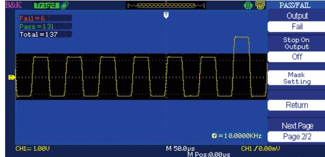
Generate user-defined pass/fail limits to quickly identify go/no go test results.
