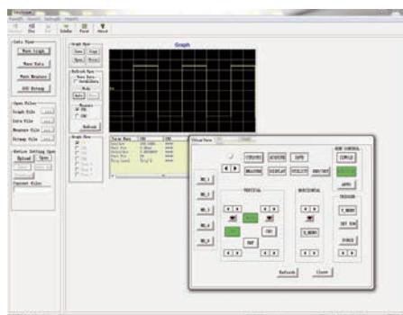
PC software is provided (free download at B&K Precision's website at [www.bkprecision.com](http://www.bkprecision.com)) for seamless integration between the oscilloscope and PC. Capture and transfer waveforms, screen images, setups and measurement results to a Windows PC via the USB device port on the back of the instrument. A USB host port on the front and rear allows for quick and easy screen saving.
