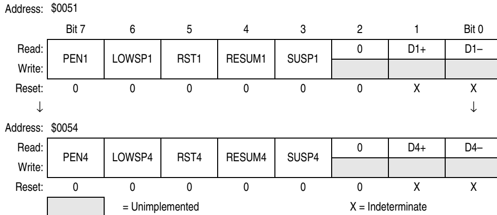
Figure 9-5. USB HUB Downstream Port Control Registers (HDP1CR-HDP4CR)
