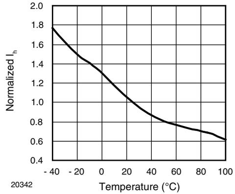
Fig. 6 - Normalized Holding Current vs. Temperature
