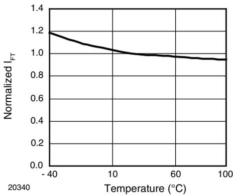
Fig. 4 - Normalized Trigger Current vs. Temperature
