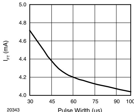
Fig. 8 - Trigger Current vs. Pulse Width
