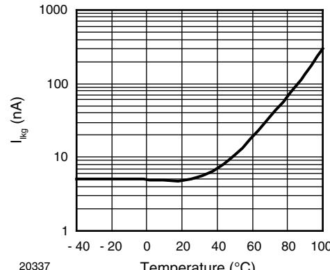
Fig. 2 - Off-State Leakage Current vs. Temperature
