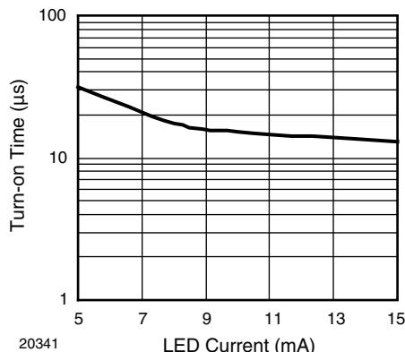
Fig. 5 - Turn-on Time vs. LED Current
