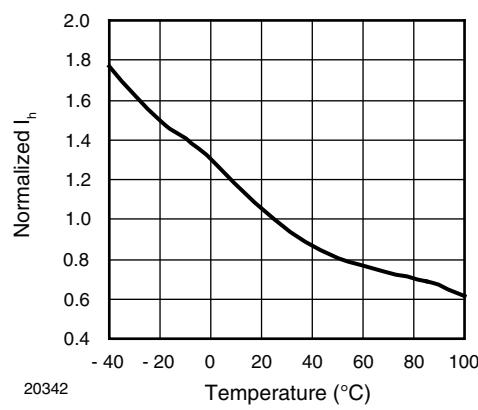
Fig. 6 - Normalized Holding Current vs. Temperature
