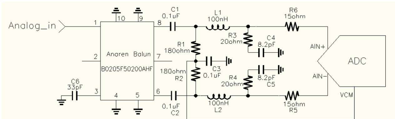
ADC frontend schematic for IF 50MHz to 110MHz
