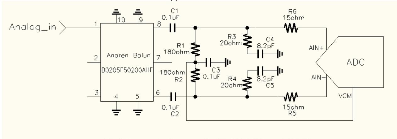
ADC frontend schematic for IF 100 MHz to 250MHz
