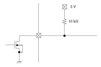
The ALERT pin is an open drain output pin. When the output pin is pulled up to the VCC with a resistor, the Low is outputted (MOSFET ON) at the Reset, and the High (internal Hi-Z) is outputted at the non-reset.
