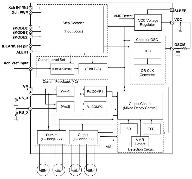
Note: Though pin functions are different depending on the used mode, they are indicated according to the  $DC(S) \times 4$  mode in this document.
