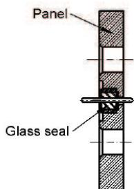
2. Place the receptacle and pre-assemble screw on the package.
