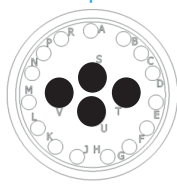
16-19* Service rating 1 15 Contacts, Size 20 4 Contacts, Size 16
