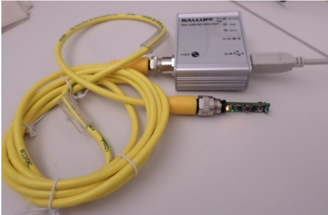
Figure 1. MAXREFDES27# Board Connected to a Balluff USB IO-Link Master
