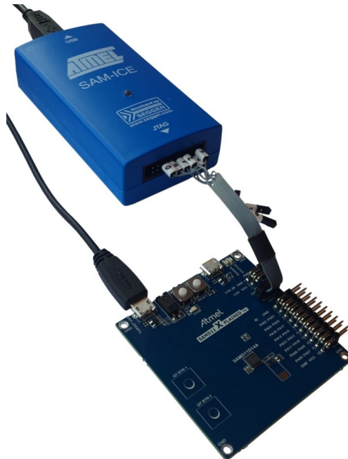
Figure 7-6. SAM-ICE using a Squid Cable
