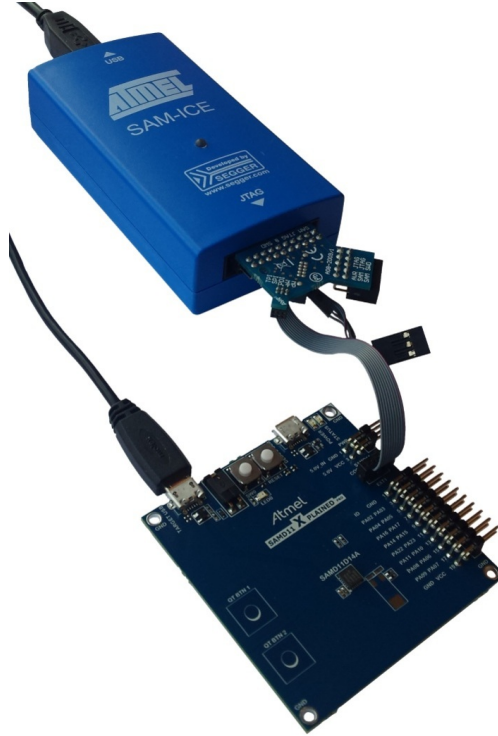
Figure 7-7. SAM-ICE using an Atmel-ICE Adapter
