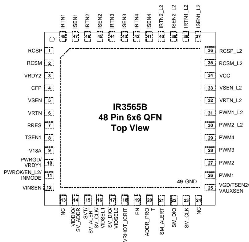
Figure 1: IR3565B Pin Diagram Enlarged
