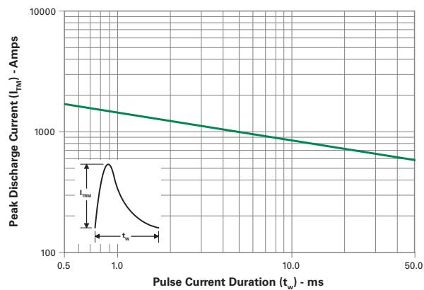
**Figure 11: Peak Capacitor Discharge Current Derating**
