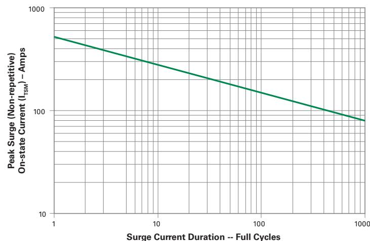
SUPPLY FREQUENCY: 60 Hz Sinusoidal
