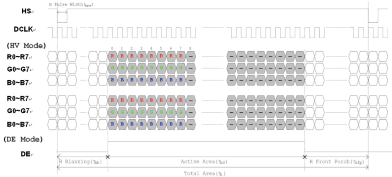
Figure 5: Horizontal Input Timing Diagram
