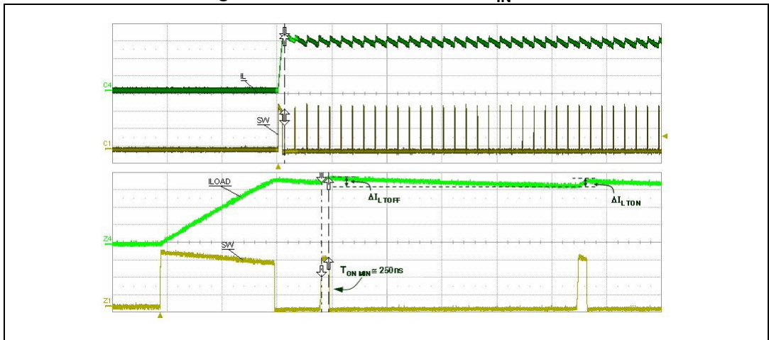
Figure 20. Short-circuit current V_{IN} = 24\text{ V}
