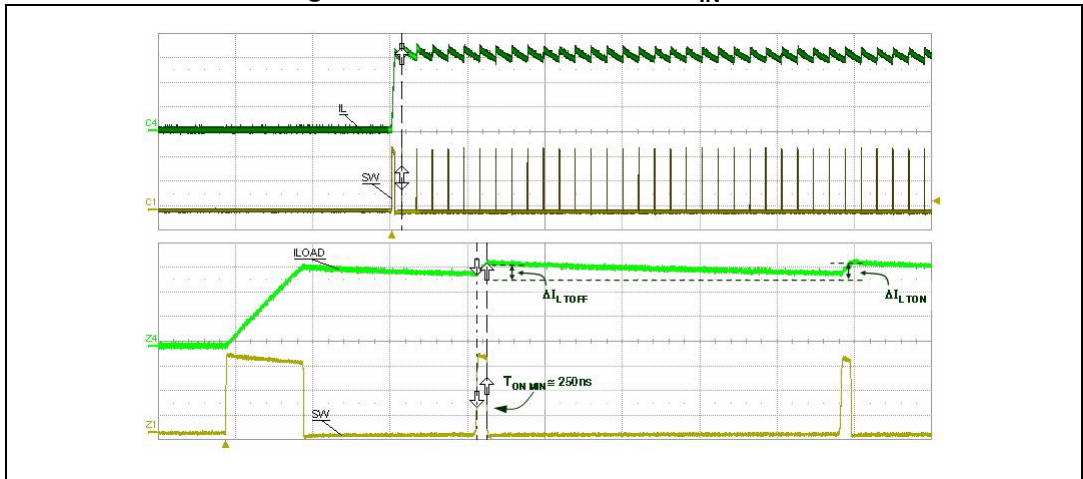
Figure 21. Short-circuit current V_{IN} = 36\text{ V}
