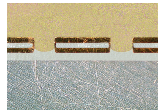
Henkel has the ability to laminate heavy copper up to 5 oz. (175µm) finished on the internal layer utilizing a thicker deposit of HT dielectric.
