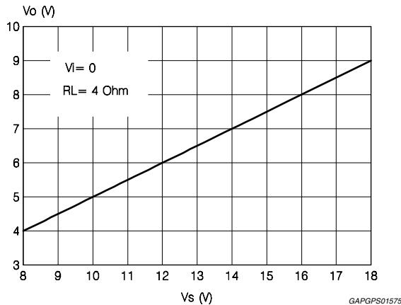
**Figure 7. Quiescent output voltage vs. supply voltage**
