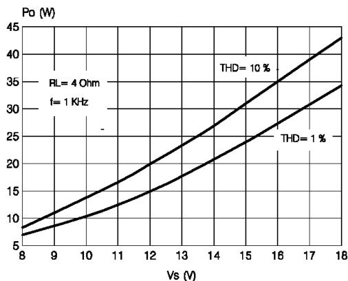
**Figure 9. Max. output power vs. supply voltage**
