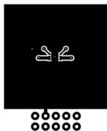
a. 57 °C/W when mounted on a 1 in 2 pad of 2 oz copper
