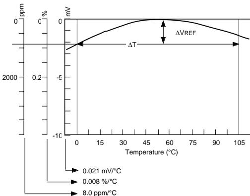
• TC in mV/°C =  $\frac{\Delta V_{REF}}{\Delta T_A}$  (mV)
