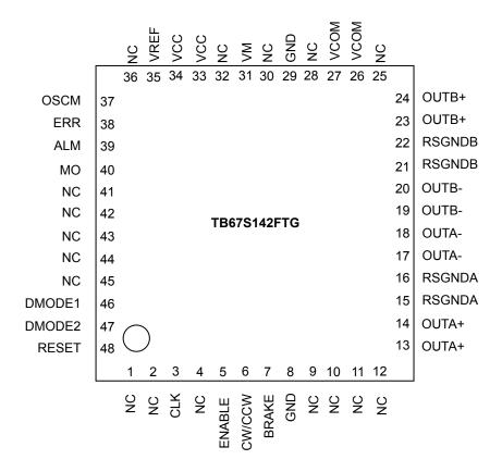
Please mount the four corner pins of the QFN package and the exposed pad to the GND area of the PCB.
