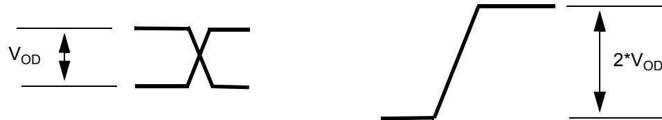
Figure 19 - Differential Voltage Parameter
