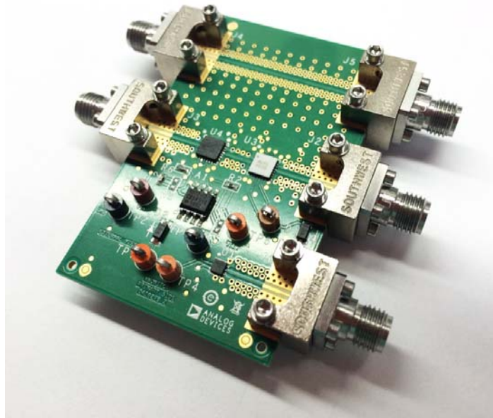
Figure 2. EVAL-CN0390-EB1Z AGC Printed Circuit Board (PCB) Photo
