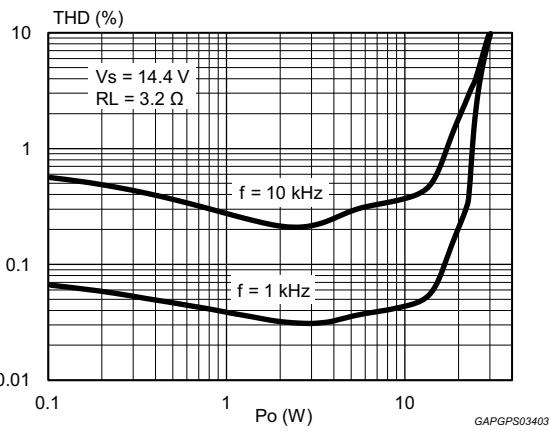
**Figure 12. Distortion vs. frequency ( $R_L = 3.2 \Omega$ )**
