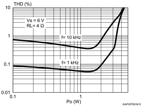
**Figure 18. Distortion vs. frequency ( $R_L = 4 \Omega, V_s = 6 \text{ V}$ )**
