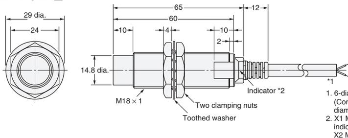
1. 6-dia. vinyl-insulated round cable with 2 conductors (Conductor cross section: 0.5 mm<sup>2</sup>, Insulator diameter: 1.9 mm), Standard length: 2 m
