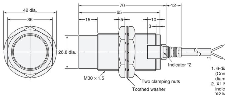
1. 6-dia. vinyl-insulated round cable with 2 conductors (Conductor cross section: 0.5 mm<sup>2</sup>, Insulator diameter: 1.9 mm), Standard length: 2 m
