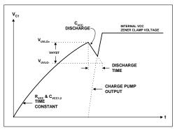
Figure 2: VCC supply voltage.
