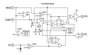
Figure 7: IRS2548D detailed PFC control circuit.
