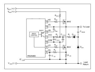
Figure 1: Start-up and supply circuitry.
