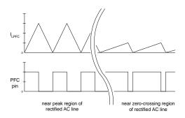
Figure 9: On-time modulation circuit timing diagram
