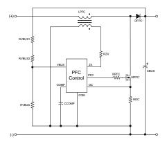
Figure 6: IRS2548D simplified PFC control circuit.
