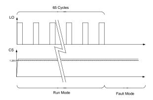
Figure 3: Fault counter timing diagram.
