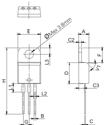
Note: Maximum torque to be applied to mounting tab is 3 in-lbs (0.3Nm).
