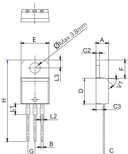
Note: Maximum torque to be applied to mounting tab is 7 in-lbs. (0.8 Nm).
