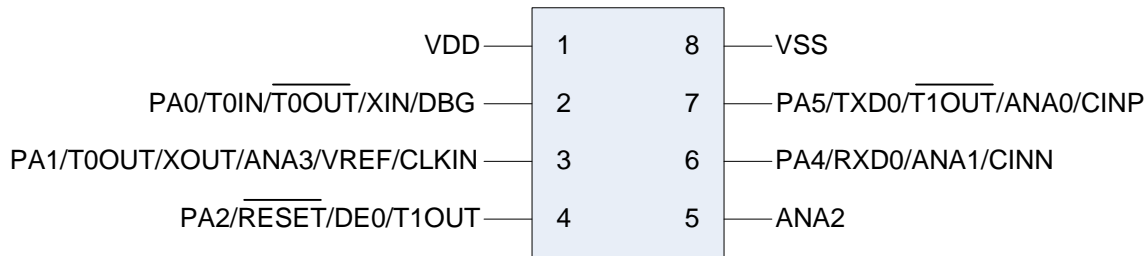
Figure 2 – 8 Pin SOIC Package Pin-Out – Z8FS040xSB20EG
