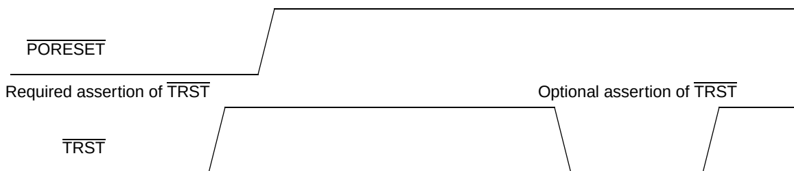
Figure 62. \overline{\text{PORESET}} vs. \overline{\text{TRST}}
